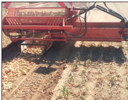
Windrow & side discharge
